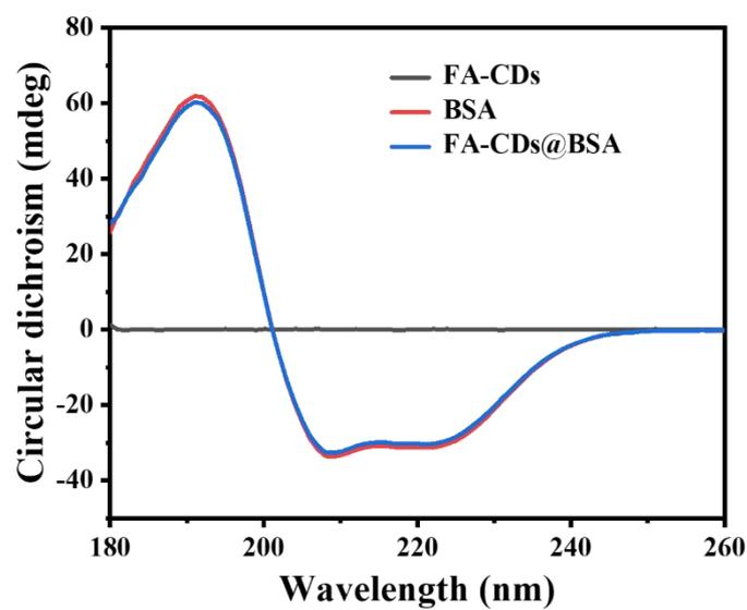
**Figure S2.** The circular dichroism spectra of FA-CDs ( $0.002 \text{ mg mL}^{-1}$ ), BSA ( $0.2 \text{ mg mL}^{-1}$ ) and FA-CDs@BSA (FA-CDs:  $0.002 \text{ mg mL}^{-1}$ , BSA: $0.2 \text{ mg mL}^{-1}$ ) in aqueous solutions.
