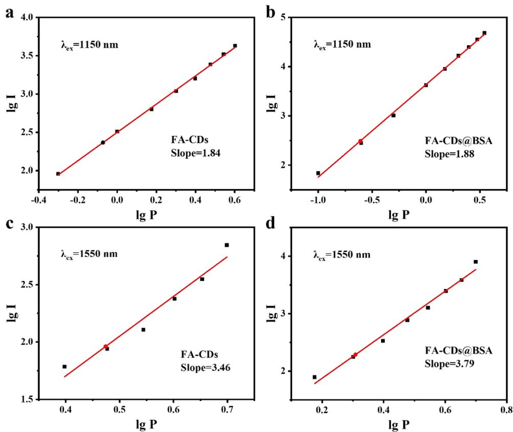
**Figure S1.** Plot of logarithm (a)(b) two-photon/(c)(d) three-photon emission intensities versus logarithm the laser power of FA-CDs ( $0.5 \text{ mg mL}^{-1}$ ) and FA-CDs@BSA (FA-CDs:  $0.5 \text{ mg mL}^{-1}$ , BSA:  $50 \text{ mg mL}^{-1}$ ).
