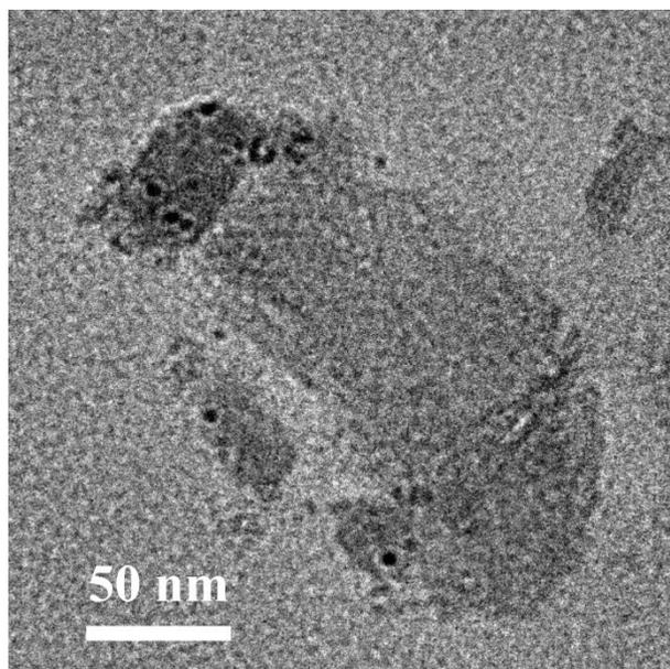
**Figure S3.** TEM image of FA-CDs@BSA (mass ratio of FA-CDs and BSA: 1:100).
